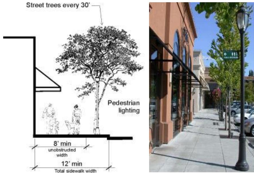
**Figure 20. Internal walkway standards and an example along retail or mixed-use buildings.**
